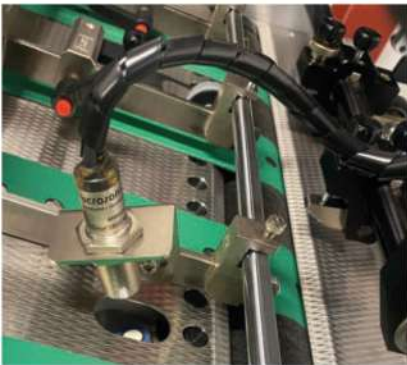
Ultra sonic double sheet detection; perfect also for very thin materials; no-set-up required.
