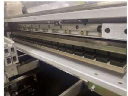
Linear electro-magnetic drive for the screen carrier R.
